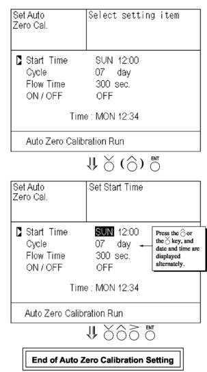
• Flow Time: The time required for purging with calibration gas.
